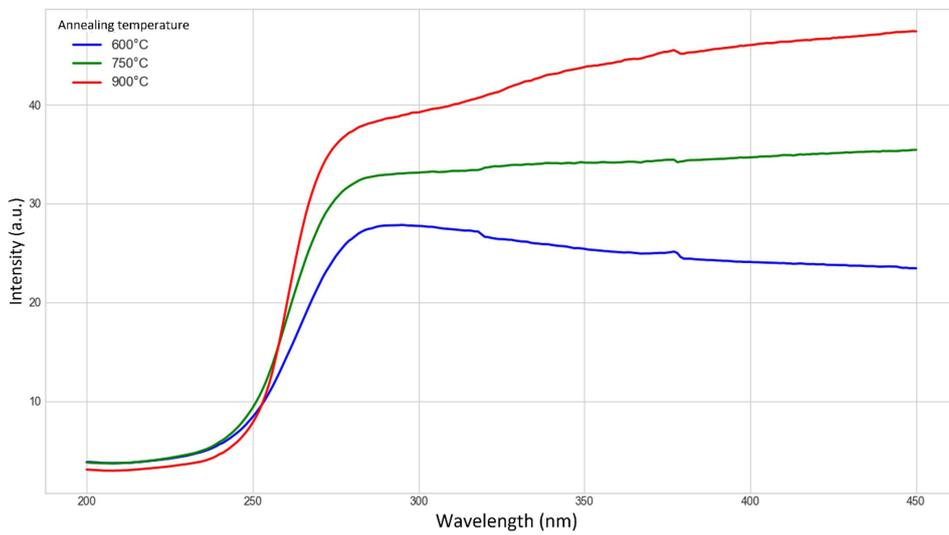
Fig. 11. Reflection spectra of obtained  $\text{Ga}_2\text{O}_3$  nanofibers.
