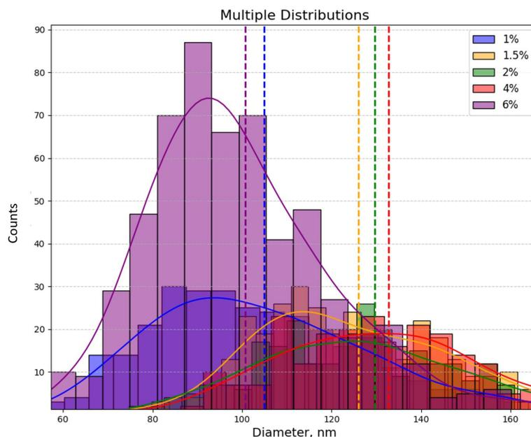
**Fig. 9.** A comparison of the diameters of annealed gallium oxide nanofibers.
