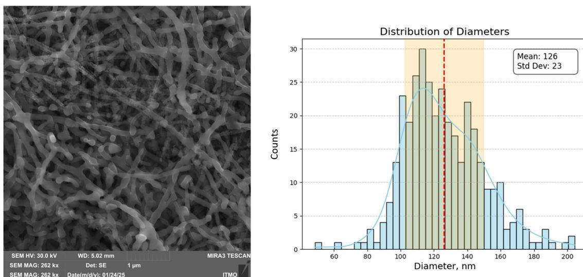
**Fig. 4.** SEM image and diameter distribution histogram of annealed nanofibers electrospun from polymer solution with 1.5 wt.% Ga. The average diameter is  $126 \pm 23$  nm.
