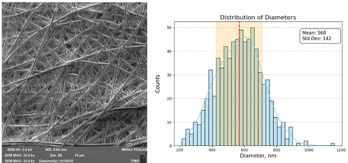
Fig. 2. SEM image and diameter distribution histogram of blank nanofibers based on PVP. The average diameter is  $568 \pm 142$  nm (mean  $\pm$  standard deviation).
