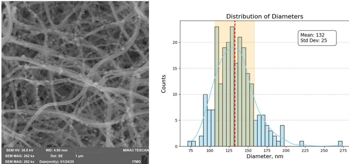
**Fig. 6.** SEM image and diameter distribution histogram of annealed nanofibers electrospun from polymer solution with 4 wt.% Ga. The average diameter is  $132 \pm 25$  nm.
