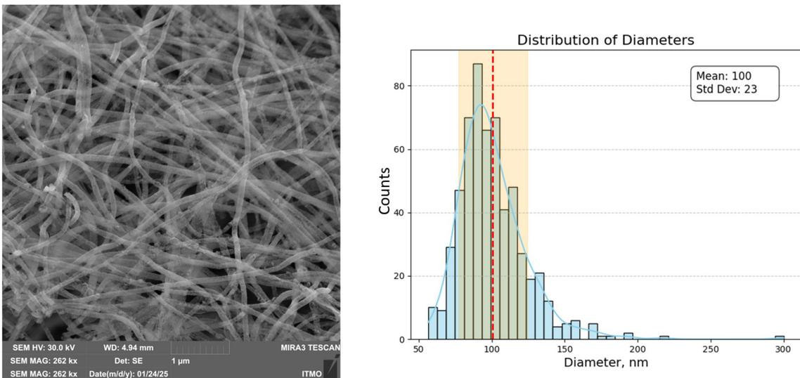
**Fig. 7.** SEM image and diameter distribution histogram of annealed nanofibers electrospun from polymer solution with 6 wt.% Ga. The average diameter is  $100 \pm 23$  nm.
