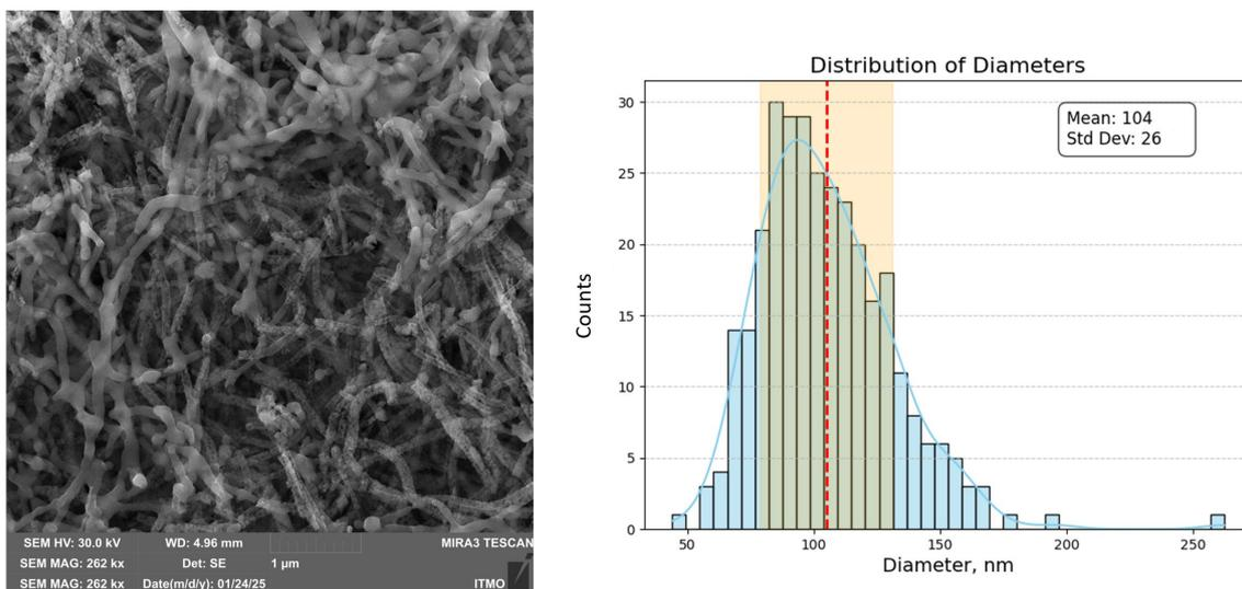
**Fig. 3.** SEM image and diameter distribution histogram of annealed nanofibers electrospun from polymer solution with 1 wt.% Ga. The average diameter is  $104 \pm 26$  nm.
