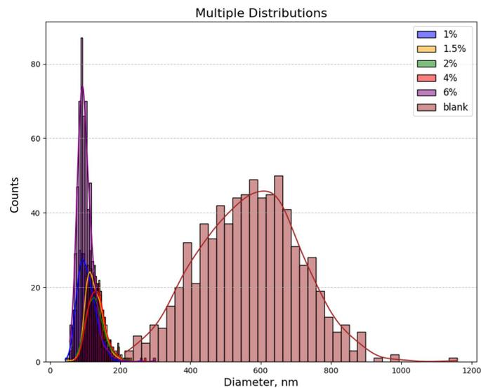
**Fig. 8.** A comparison of the diameters of annealed gallium oxide nanofibers with blank polymer nanofibers.
