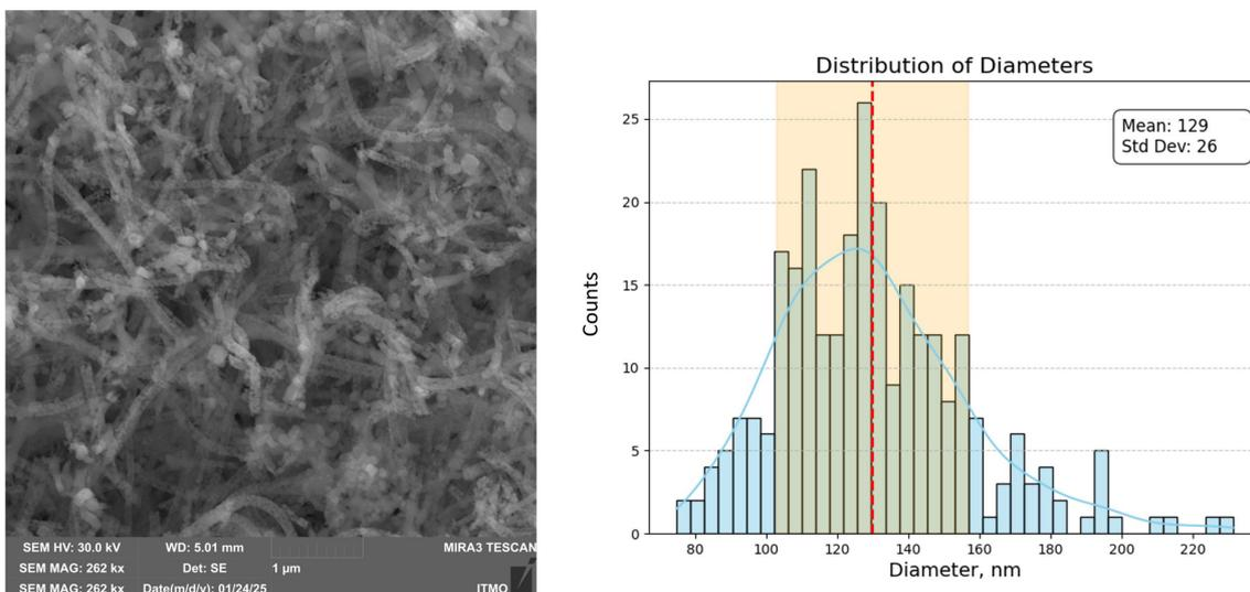
**Fig. 5.** SEM image and diameter distribution histogram of annealed nanofibers electrospun from polymer solution with 2 wt.% Ga. The average diameter is  $129 \pm 26$  nm.
