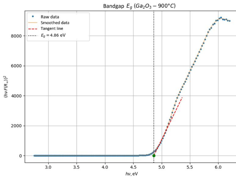
Fig. 12. The bandgap energy  $E_g$  of obtained  $\text{Ga}_2\text{O}_3$  nanofibers.
